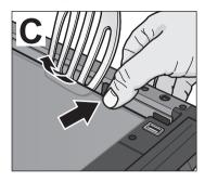
Press in the retaining clip with your thumb on one side and disengage the inner door glass e.g. with the spatula, then repeat on the other side. (Fig. C).
